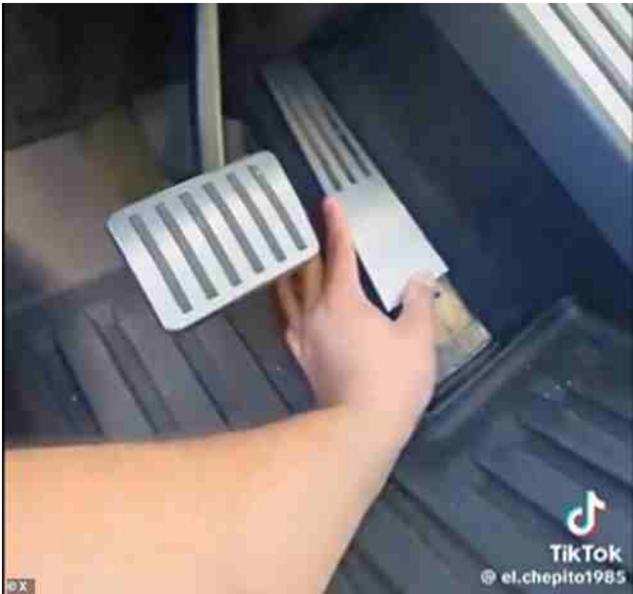
The pedal cover was wedged under a piece of fabric that was part of the vehicle's floorboard, making it impossible to the driver to release it until he was able to stop the Cybertruck
